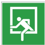
Emergency escape opening
