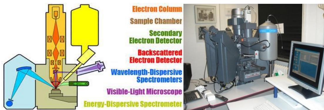
Fig. 6: Schematic picture of an EMPA [25] and a foto of Cameca electron probe micro-analyzer SX 100
